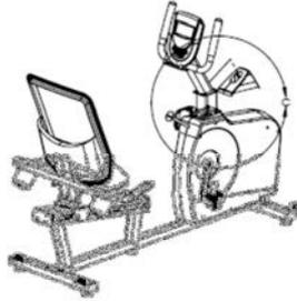
Before attaching the Mast, be sure to connect all the cables in the Mast to the appropriate cables in the frame. Once all cables are connected put the Mast over the bolts, slide into position and tighten the bolts. Make sure the cables are securely put away and do not get pinched.
